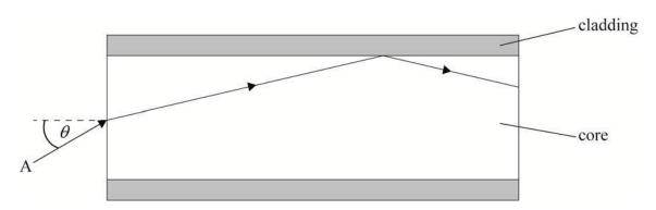
refraction angle on entering core sensible and smaller than incidence angle; equal angles of reflection at cladding; (judge by eye)
